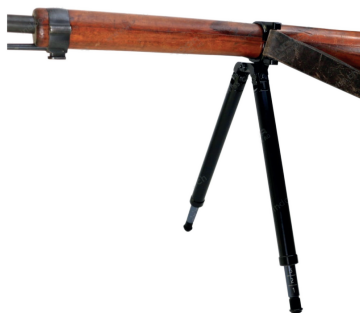
Figure 27: Bipied réglable Wyss
